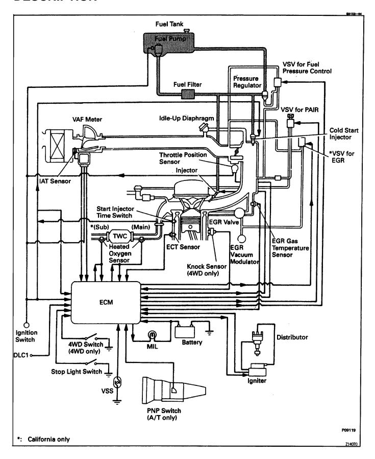
The MFI system is composed of three basic subsystems: Fuel, Air Induction and Electronic Control Systems.
