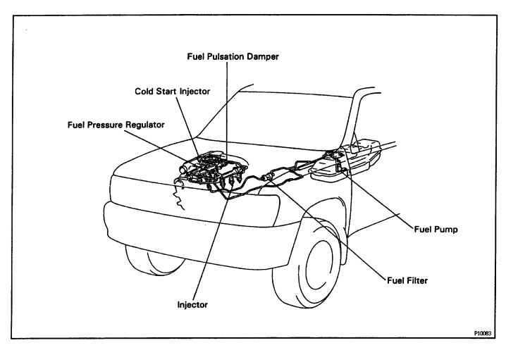
Fuel pumped up by the fuel pump flows through the fuel filter and is distributed to each injector and cold start injector at a set pressure maintained by the fuel pressure regulator.
