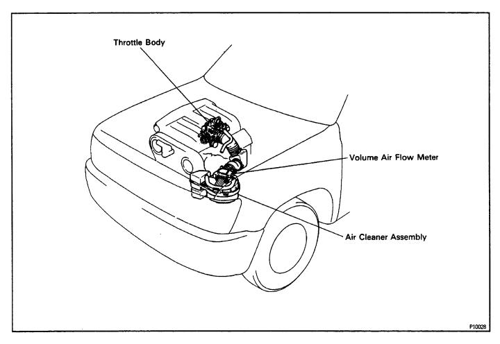
Air filtered through the air cleaner passes through the volume air flow meter and the amount flowing to the air intake chamber is determined according to the throttle valve opening in the throttle body and the engine speed.
