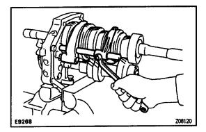
(c) Install the shift fork No.2 with a new bolt and torque the bolt.
