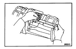
(e) Install the shift lever shaft to the transfer adaptor and shift lever housing.
