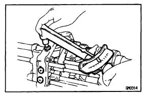
(b) Apply sealant to the plug threads.
