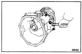
(d) Install the shift lever housing to the transfer adaptor and connect the fork shafts.
