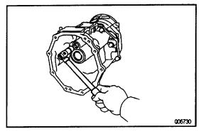
(g) Using a hexagon wrench, install and torque the plug. Torque: 37 N-m (380 kgf-cm, 27 ft-lbf)
