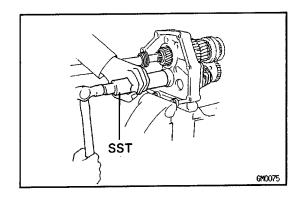
(b) Install the counter gear into the intermediate plate while holding the counter gear and install a new counter rear bearing with SST. SST 09316–60010 (09316–00010)
