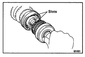
(b) Install the input shaft to the output shaft with the synchronizer ring slots aligned with the shifting keys.
