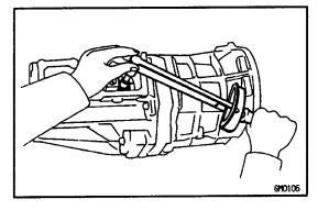
(f) Install and torque the shift lever housing set bolt. Torque: 38 N-m (390 kgf-cm, 28 ft-lbf)
