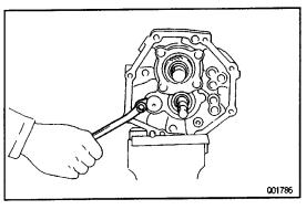
(b) Install the shaft stopper and torque the bolt.
