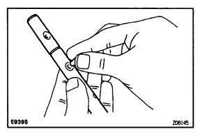
(c) Apply MP grease to the interlock pin No.2 and install them into the shift fork shaft No.3.
