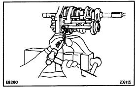
(f) Using a pin punch and hammer, drive in the slotted spring pin.
