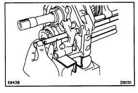
(h) Install the shift fork shaft No.5 through the reverse shift head and intermediate plate.
