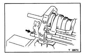
(g) Install the shift fork No.3 with a new bolt and torque the bolt.
