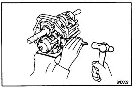
(i) Using a pin punch and hammer, drive in the slotted spring pin to the reverse shift head.
