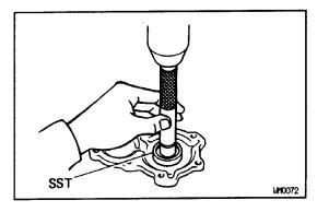
(b) Using SST and a press, press in a new oil seal. SST 09223–50010
