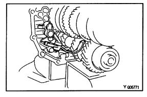
(b) Install the reverse shift arm to the pivot of the reverse shift arm bracket.
