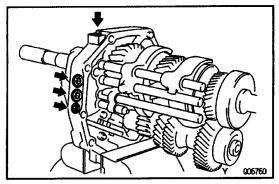
(c) Using a hexagon wrench, torque the 4 screw plugs.
