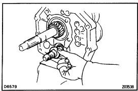
8. INSTALL STRAIGHT PIN AND THRUST WASHER
