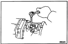
(f) Install and torque the shift lever housing set bolt.
