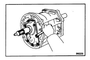
(c) Apply sealant to the bolt threads.
