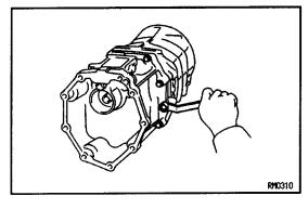
(e) Install and torque the 10 bolts.
