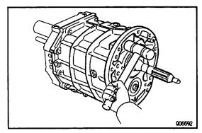
(c) Align the 2 bearing outer race, 3 fork shaft end and reverse idler gear shaft end with the case installation holes, and install the case.
