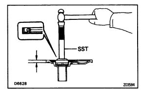
(b) Using SST and a hammer, drive in a new oil seal. SST 09608 - 35014 (09608 - 06020, 09608 -06090)
