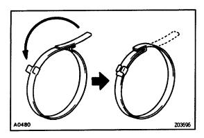
(c) Bend the band and lock it, as shown in the illustration.
