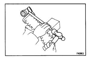
(c) Using a brass bar and hammer, remove the tripod joint from the drive shaft.
