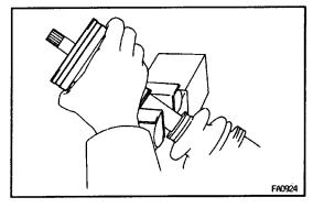
3. TEMPORARILY INSTALL NEW BOOT AND NEW BOOT CLAMPS FOR INBOARD JOINT TO DRIVE SHAFT
