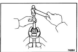
(c) Using a brass bar and hammer, tap in the tripod joint onto the drive shaft.
