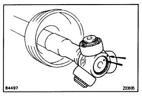
(b) Align the matchmarks placed before disassembly.
