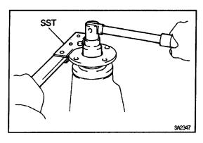
(c) Adjust the drive pinion preload by tightening the companion flange nut.
