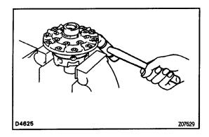
(c) Using a plastic hammer, separate the LH and RH cases.
