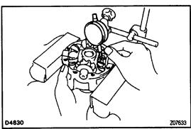
(e) Hold the side gear, measure the side gear backlash.
