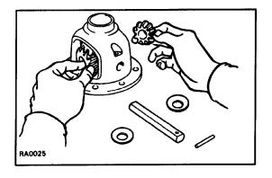
(b) Install thrust washers and side gears in the differential case.
