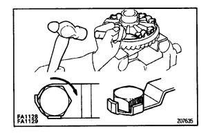
Using a hammer and drift punch, stake the lock plates. HINT: Stake 1 claw flush with the flat surface of the bolt. For the claw contacting the protruding portion of the bolt, stake only the half portion of the tightening side.
