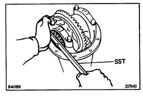
(c) Using SST, tighten the adjusting nut on the ring gear side until the ring gear has a backlash of about 0.2 mm (0.008 in.).
