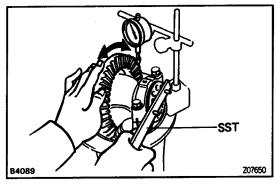
(h) Using a dial indicator, adjust the ring gear backlash within specification.
