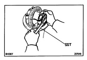
(g) Tighten the adjusting nut 1 - 1.5 notches from the zero preload position.
