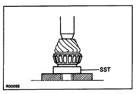
(b) Using SST and a press, press the reused washer and new rear bearing on the drive pinion.
