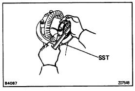
(d) While turning the ring gear, use SST to fully tighter the adjusting nut on the drive pinion side. After the bearing are settled, loosen the adjusting nut on the drive pinion side.
