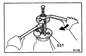
(b) Install the companion flange with the SST. SST 09950–30010
