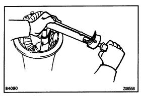
(i) Torque the bearing cap bolts.
