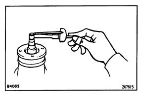
(k) Using a torque wrench, measure the total preload.
