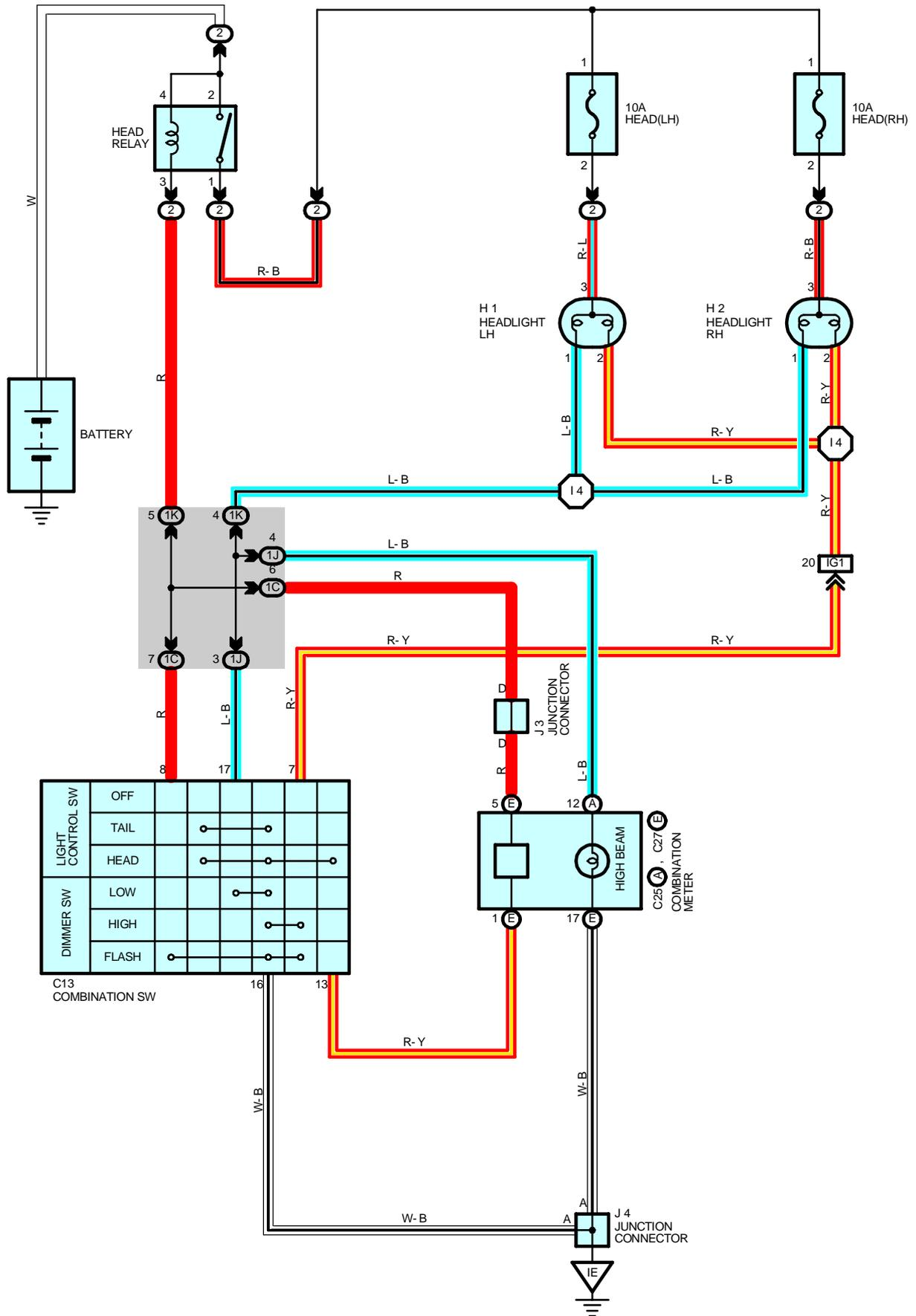
**SERVICE HINTS****HEAD RELAY**2-1 : Closed with light control SW at **HEAD** position or dimmer SW at **FLASH** position
